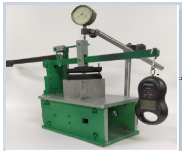
Figure 7: Portable lever press with a stand mounted on it for transverse compression of the PA trunk.
